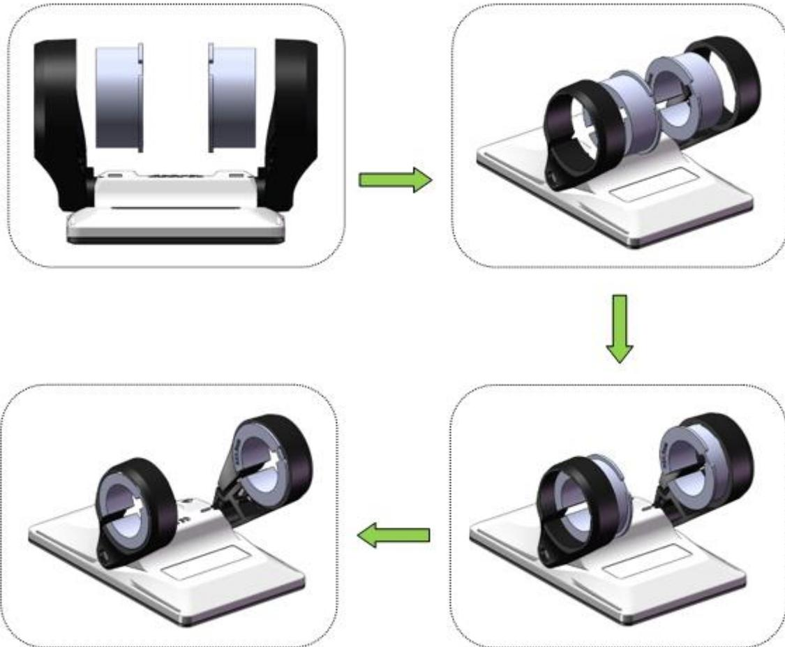
Note: The installation direction of the adjusting washer must be from the inside to the outside of the bracket.
