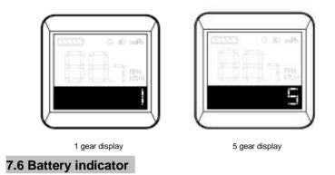
Five segments all are on when at full state. When it is at low voltage, the last segment will flash to warn .
